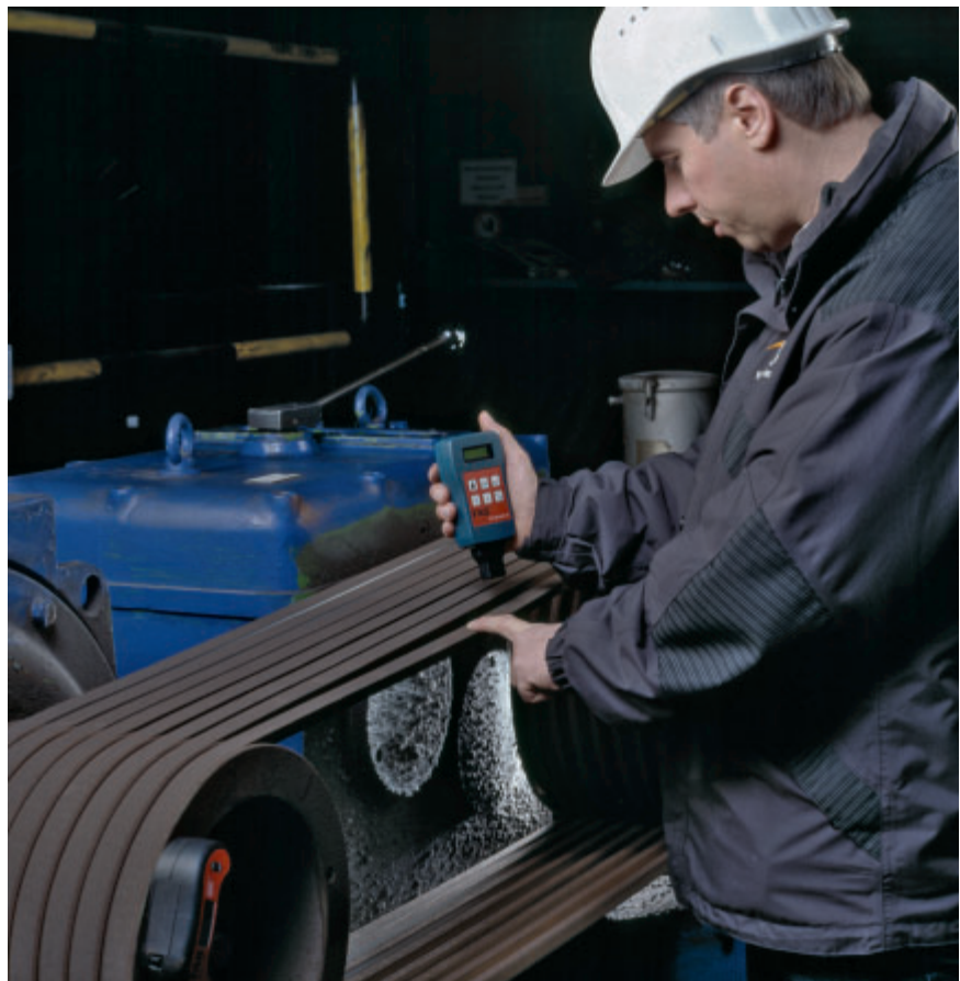
Measurement using cableless measurement probe
