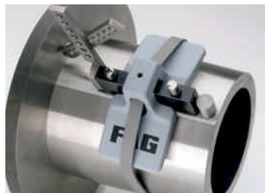
Figure 5: Taper measuring instrument attached to the side of a journal
